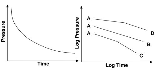
is expected to be a straight line (like line A-B). A change to a steeper slope (line A-C) indicates leakage in the system; initial flatter slope (line A-D) indicates air entrapment at the start of the test.
